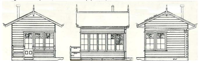
A drawing of the model. The non-door end wall has two (2) windows, model has three (3).
